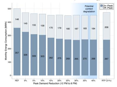
In the real-time price (RTP) case, QCo substituted a block & index hourly electric price for the flat electric price, and removed all peak demand charges. Operations were optimized to minimize energy expense, and the building achieved a 21% peak reduction as a byproduct. This is not an unexpected result – QCo algorithms avoided high hourly electric prices, which typically occur during peak demand periods.
